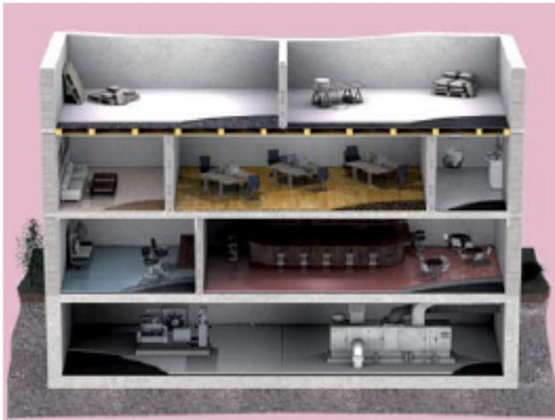
**Damtec® impact sound reduction products are suitable for use directly under flooring, under screed or on a wooden sub-floor.**
